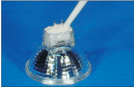
Production Potting of High Performance Light Bulbs
