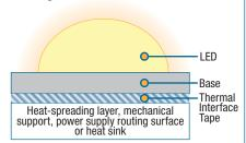
**Durability of interface:** Especially in external applications of LEDs, durability of the thermal interface is important to support efficiency in different environmental conditions. 3M products have shown excellent durability through accelerated aging tests.
