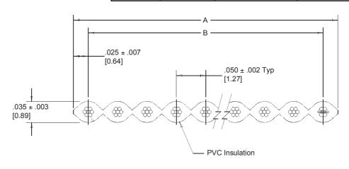
28 AWG, 7 X 36 [ 7 X ø 0.127 ] Tinned Stranded Copper Conductors
