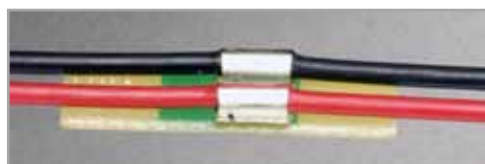
Figure 3: Wires Properly Terminated by the Press
