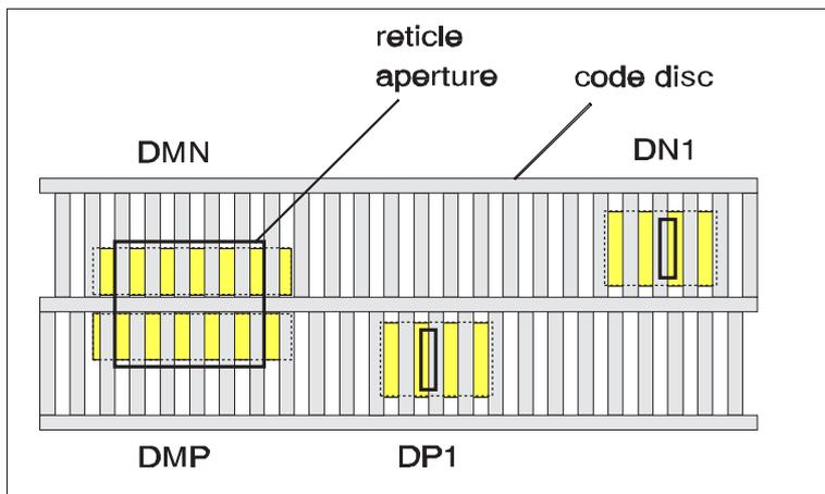
Figure 3: Position monitoring with photodiodes DMP, DMN
