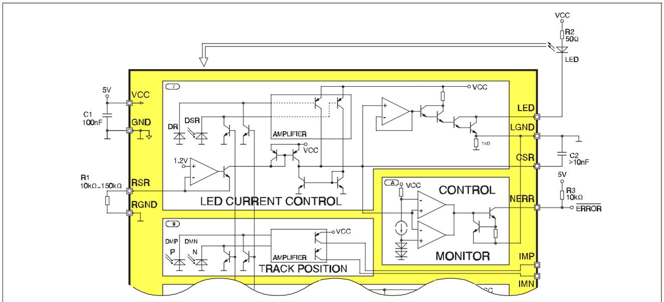
Figure 1: LED current control and control monitor
