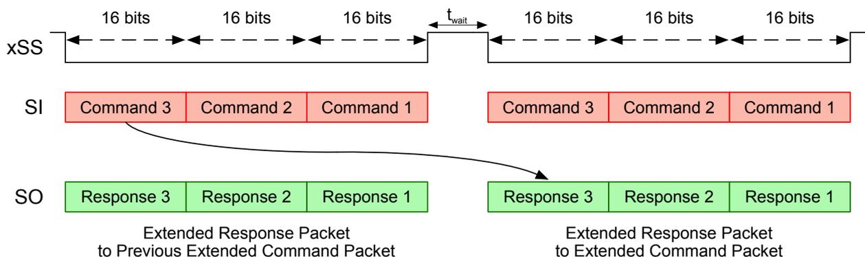
Figure 11: Extended communication packet structure with chained iC-TW11s
