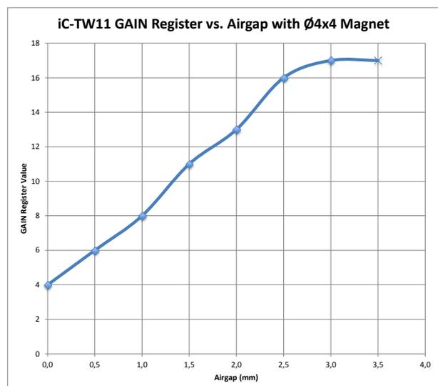
Figure 8: Typical Hall array gain vs. airgap
