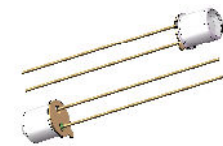
TO46-2L1 Ø 4.7 mm, h 5.39 mm RoHS compliant
