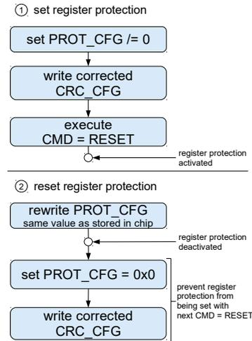
Figure 39: Enabling/disabling register protection
