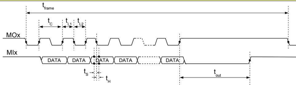
Figure 7: Multiturn SSI Interface Timing (x = 1, 2; MODE\_MT = 0x0..0x5, 0x8..0xD)
