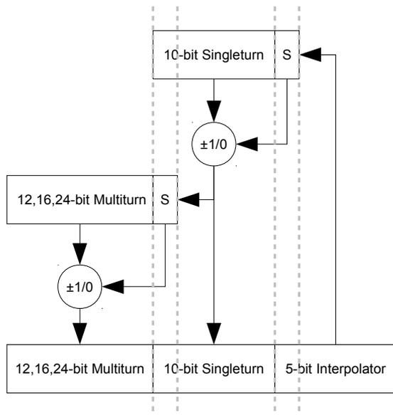
Figure 40: Synchronization position value
