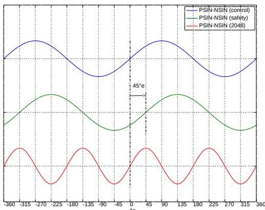
Figure 10: Sine/Cosine phase-shift, °e = with reference to one electrical period
