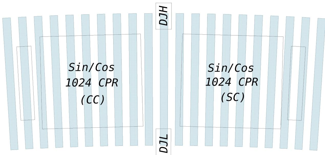
Figure 46: Alignment diodes DJH, DJL for radial alignment
