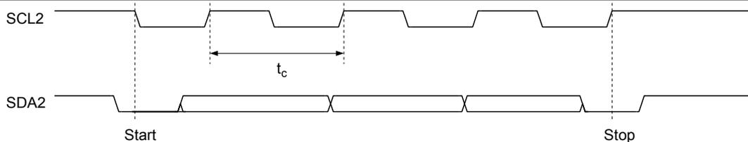
Figure 8: I<sup>2</sup>C Timing
