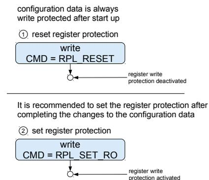
Figure 36: Setting/resetting register protection
