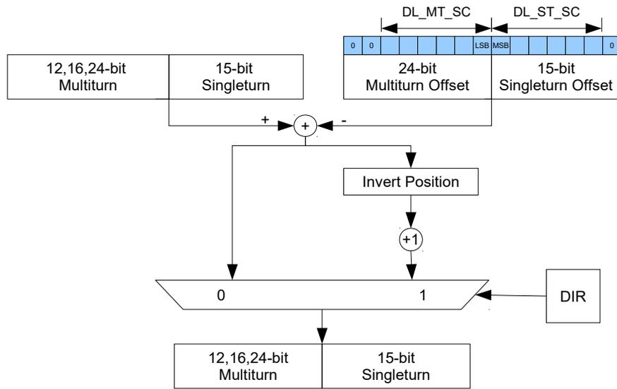
Figure 41: Offset and code direction calculation (Safety Channel only)
