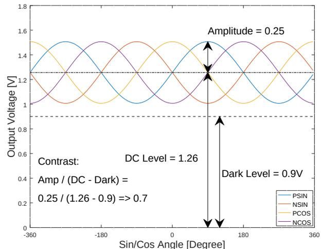
Figure 13: Signal level for contrast 70%
