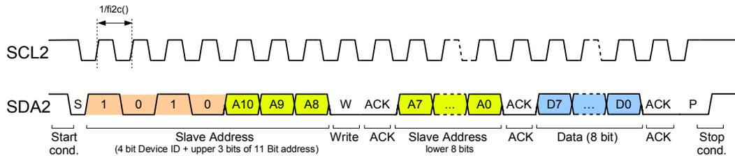
Figure 18: Example of line signals for I2C protocol: write single byte to EEPROM. The second part of the slave address (lower 8 bits) is representing the register address.
