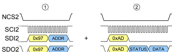
Figure 24: Read Register: set the read address (1) + opcode REGISTER status/data to read-out data (2)
