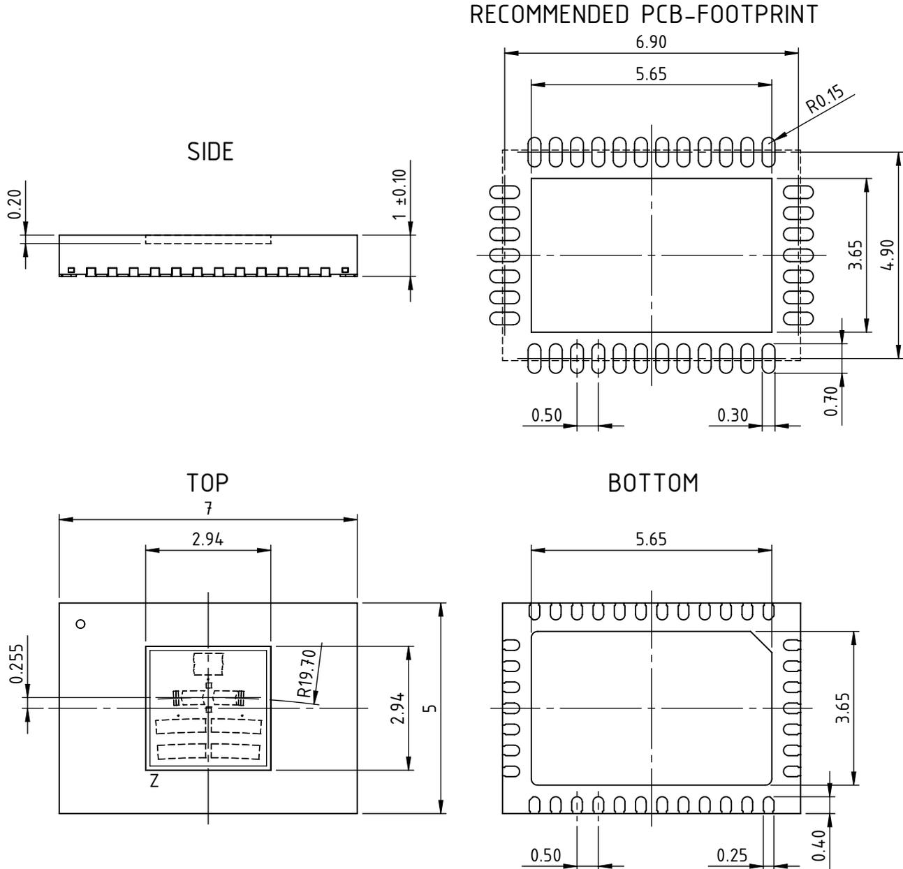
All dimensions given in mm. General tolerances of form and position according to JEDEC MO-220. Positional tolerance of sensor pattern:  $\pm 70\mu\text{m}$  /  $\pm 0.6^\circ$  (with respect to center of backside pad). Maximum molding excess  $+10\mu\text{m}$  /  $-75\mu\text{m}$  versus surface of glass. Small pits in the mold surface, which may occasionally appear due to the manufacturing process, are cosmetic in nature and do not affect reliability.
