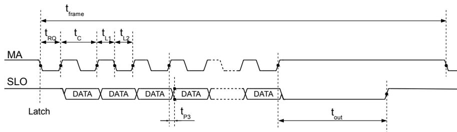
Figure 4: SSI Protocol Timing (SC: IF\_MODE = 0x2, 0x3).
