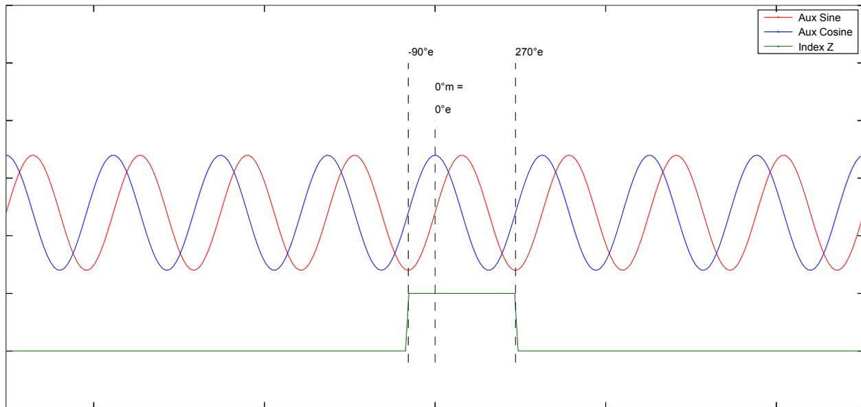
Auxiliary sine/cosine with index Z pulse
