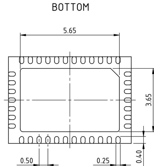
All dimensions given in mm. General tolerances of form and position according to JEDEC MO-220.
