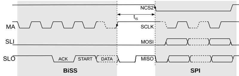
Figure 3: Switching from BiSS to SPI (SC: IF\_MODE = 0x0).
