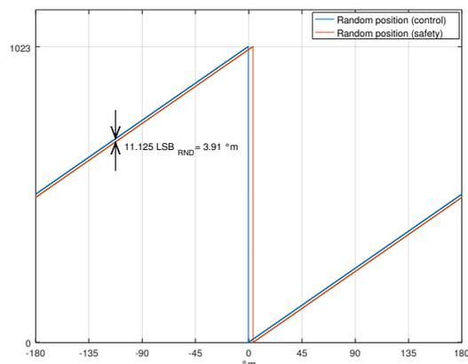
Figure 11: PRC position difference, °m = with reference to one mechanical revolution
