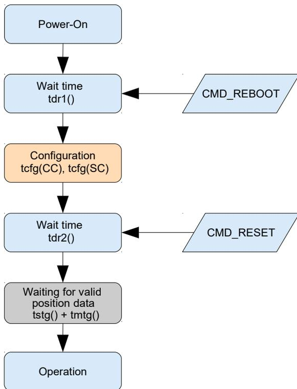
Figure 14: Overview of startup process
