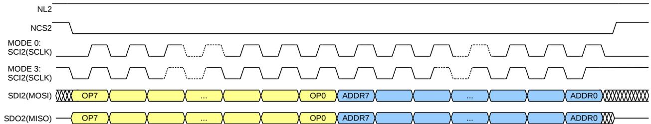
Figure 22: SPI protocol Safety Channel
