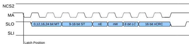
Figure 21: Extended SSI protocol
