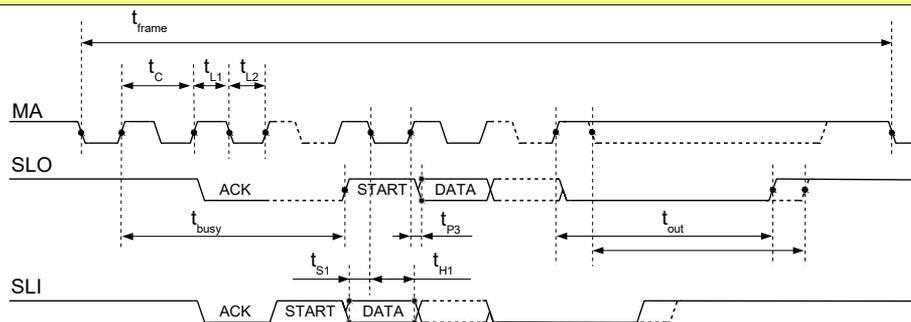
Figure 2: BiSS Protocol Timing (SC: IF\_MODE = 0x0, 0x1). Signal MA refers to input SCI2, signal SLO to output SDO2, signal SLI to input SDI2.
