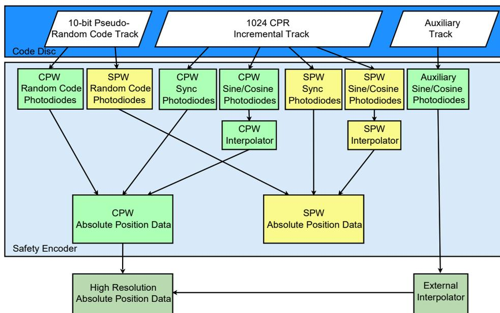
Figure 9: Principle data flow
