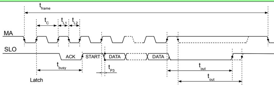
Figure 1: BiSS Protocol Timing (CC). Signal MA refers to input MA1, signal SLO to output SLO1.
