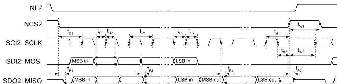
Figure 5: SPI Timing (IF\_MODE = 0x0, 0x4, 0x5)
