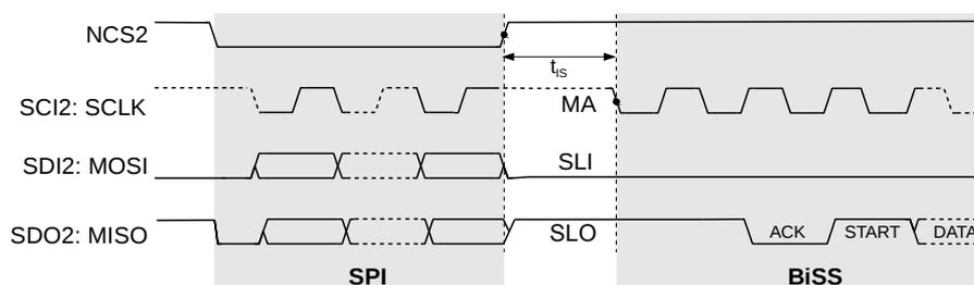
Figure 6: Switching from SPI to BiSS (IF\_MODE = 0x0)
