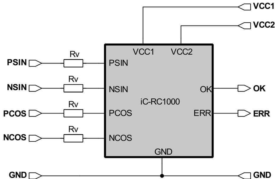
Figure 3: Overvoltage protection with external resistors
