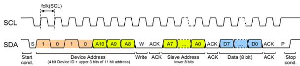
Figure 5: I<sup>2</sup>C slave addressing for writing a single byte to the EEPROM.
