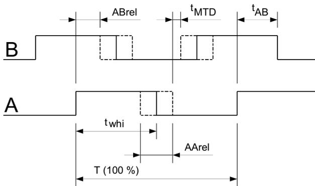
Figure 3: Relative angle error and minimum edge distance.
