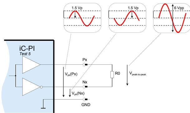
Figure 16: Definition of 6 V<sub>pp</sub> differential test signal. Termination R0 must be high-impedance (resistive) during all *Test* and *Calibration* modes.
