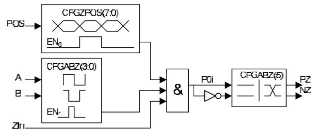
Figure 23: Signal path from  $Z_{in}$  to PZ/NZ
