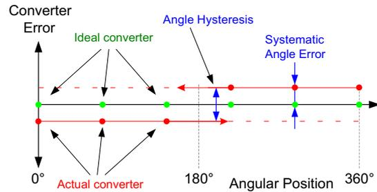
Figure 2: Systematic angle error due to hysteresis.
