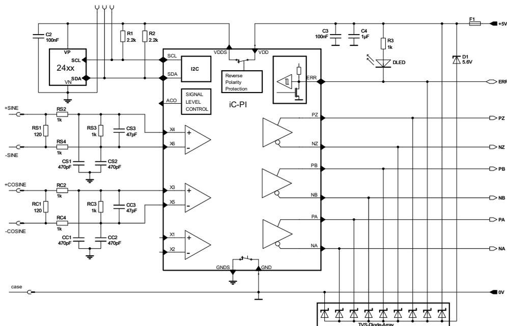
Figure 41: Input circuit for sine encoders (0.8 V<sub>pp</sub> to 1.2 V<sub>pp</sub>) with 120 Ω termination and low-pass filtering. RS2/RS4 and RC2/RC4 serve as protection against ESD and transients. RS3 and RC3 reduce the input signal levels to 1/3 suiting for an overall gain of 18 (GR12 x GF1, resp. G12 x GF2).
