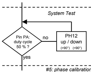
Figure 35: Correction of the sine-to-cosine phase shift by PH12. Repeating the gain and offset calibrations may be reasonable if larger phase correction values are required (refer to chapter signal conditioning for further details).
