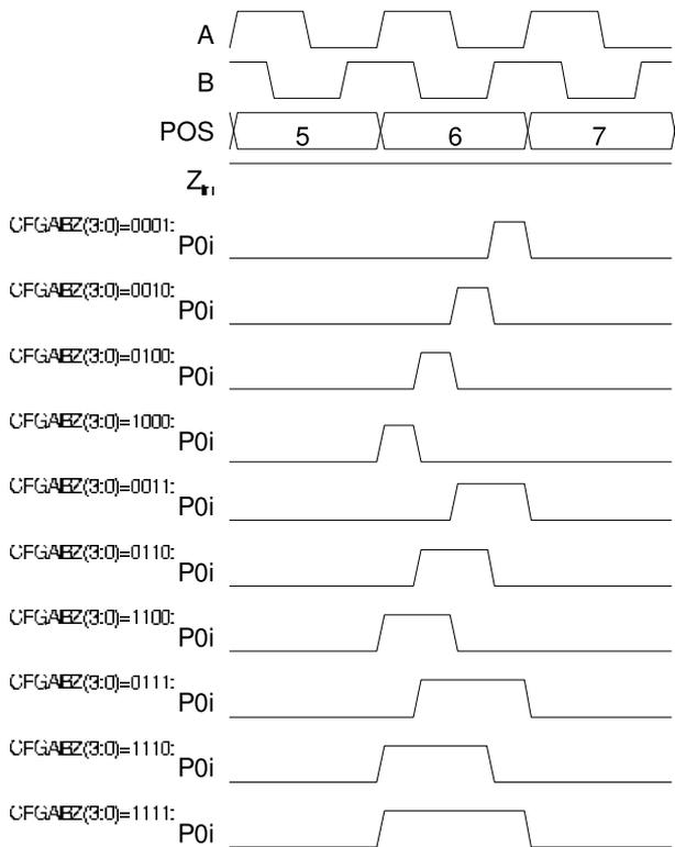
Figure 24: Zero signal gating by CFGABZ(3:0);
