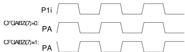
Figure 26: Function of CFGABZ(7)
