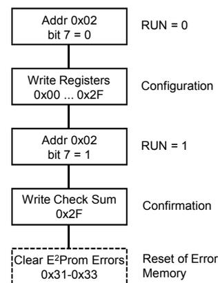
Figure 9: Programming via I<sup>2</sup>C. RUN is altered by changing only bit 7 of address 0x02 and leaving bits 6:0 unchanged.
