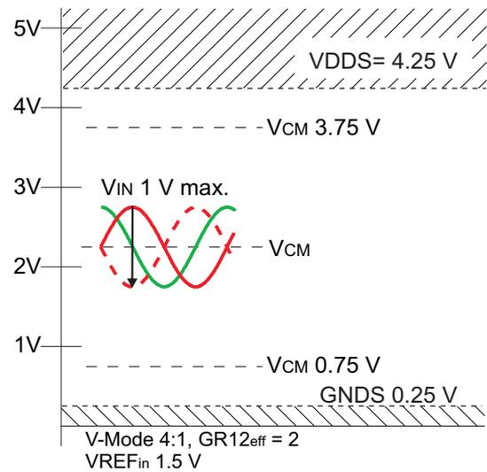
Figure 13: Permissible maximum input amplitude  $V_{IN}$  and common mode input range  $V_{CM}$  for  $G12_{eff} = 2.0$  and V-Mode 4:1.
