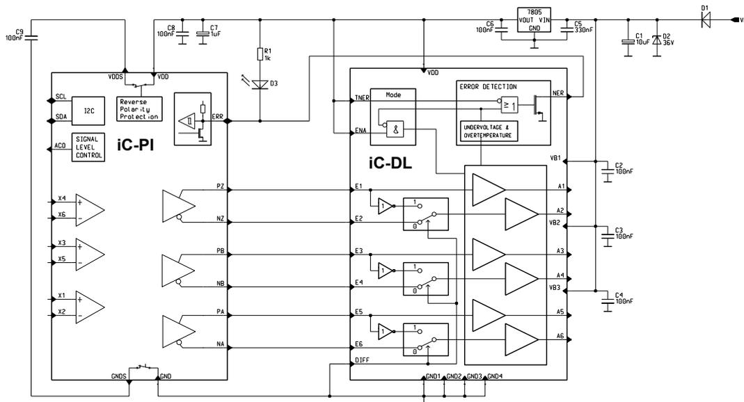
Figure 40: Application example with 24 V line driver.
