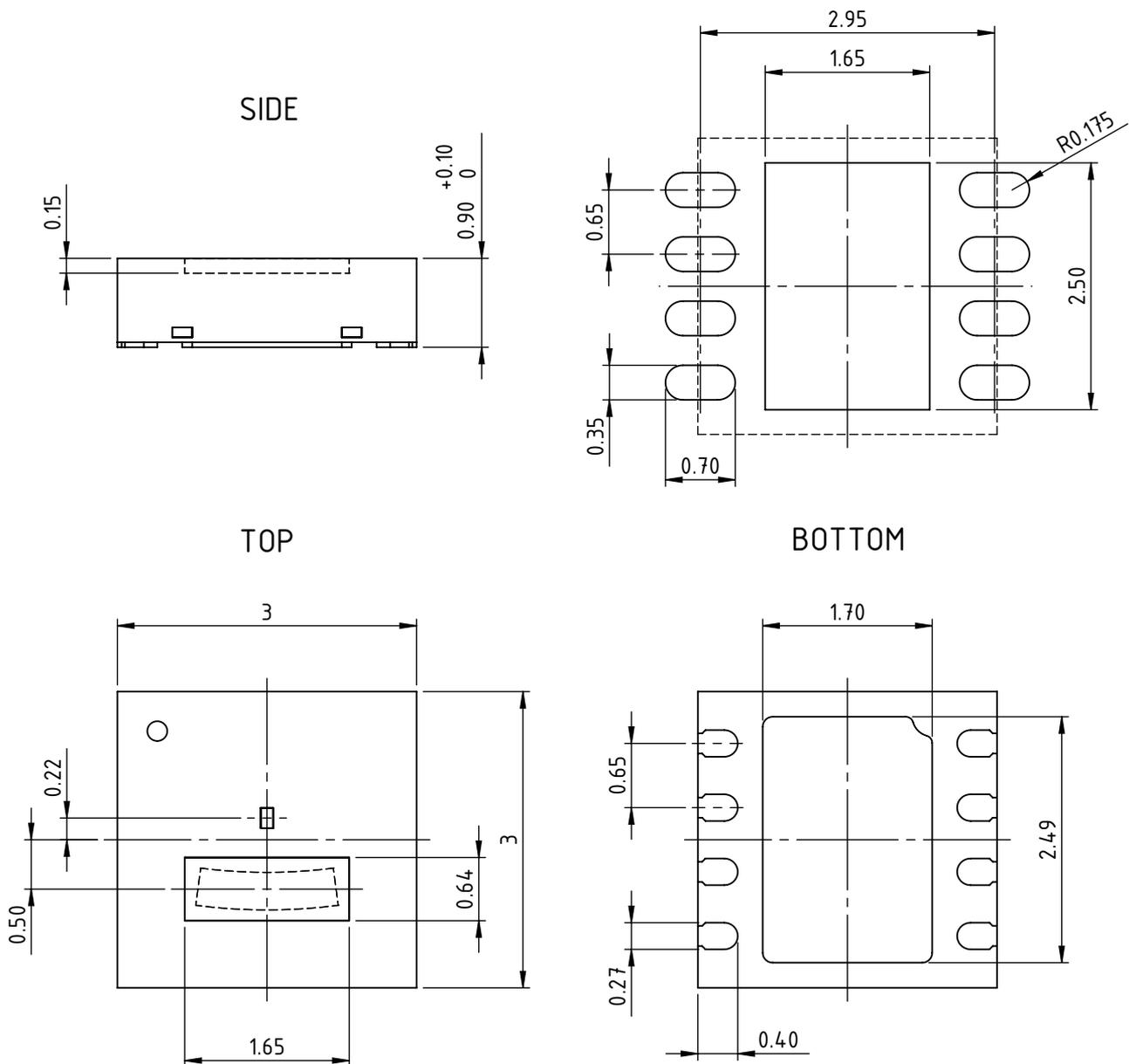
All dimensions given in mm. General tolerances of form and position according to JEDEC MO-229.
