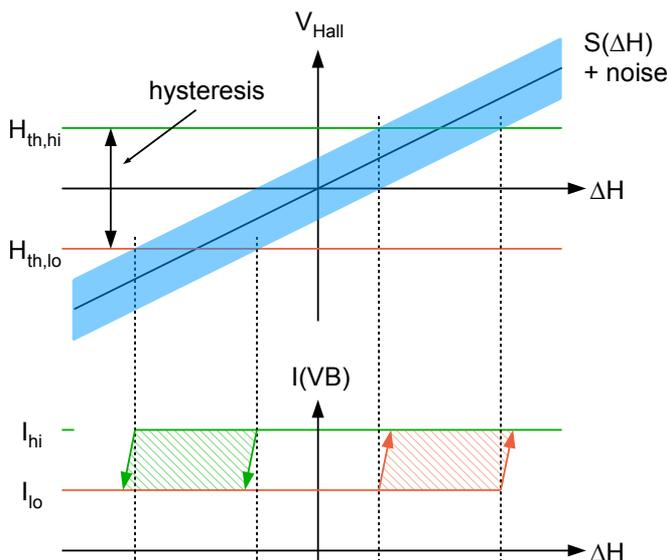
Figure 3: Switching behaviour vs. magnetic input signal
