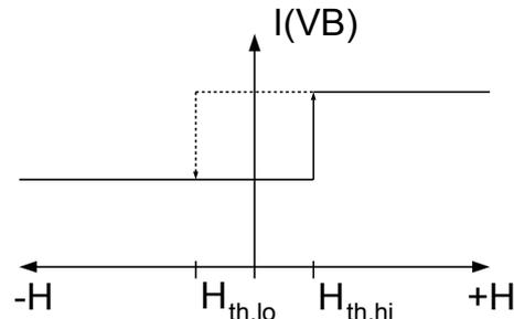
Figure 1: Current level switching vs. magnetic field difference
