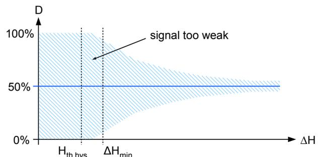
Figure 5: Duty-cycle as a function of  $\Delta H$
