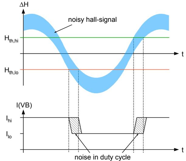
Figure 4: Effect of noise on output duty-cycle
