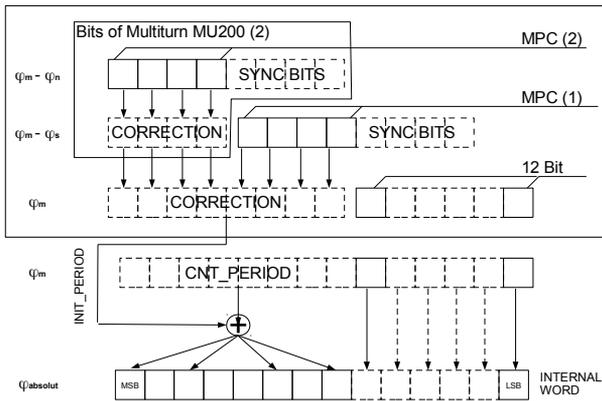
Figure 44: Principle of the synchronization of a 3-track nonius system using 2 iC-MU200 without further multitrans data
