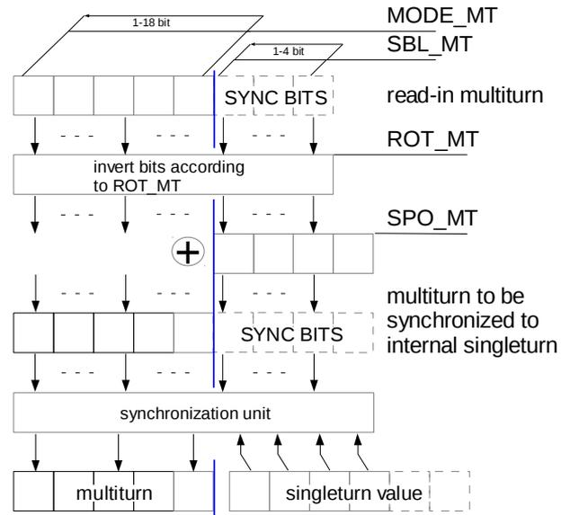
Figure 41: Parameters to configure external multiturn
