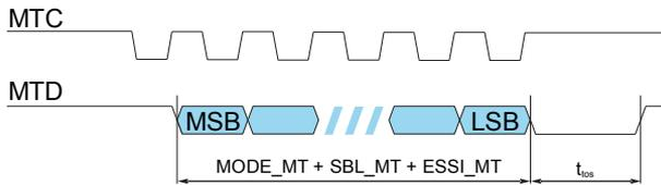
Figure 38: Example of multiturn SSI line signals
