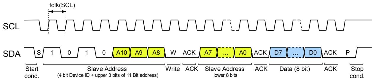
Figure 13: I<sup>2</sup>C slave addressing for writing a single byte to the EEPROM.
