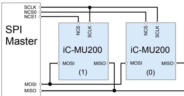
Figure 21: Example configuration SPI bus with 2 parallel Slaves
