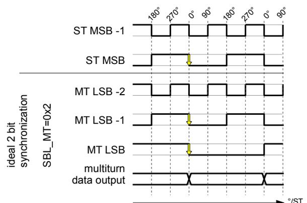
Figure 40: Principle of 2 bit MT synchronization
