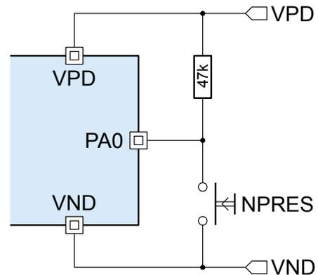
Figure 53: External circuitry for NPRES functionality
