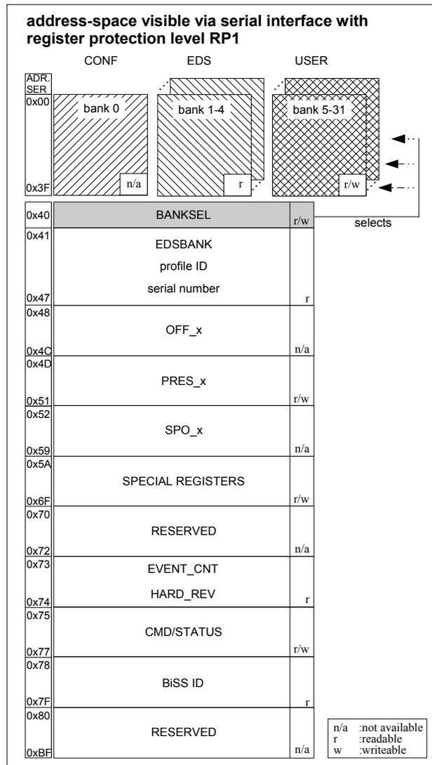
Figure 50: Principle of bank-wise memory addressing and access restrictions with register protection level RP1
