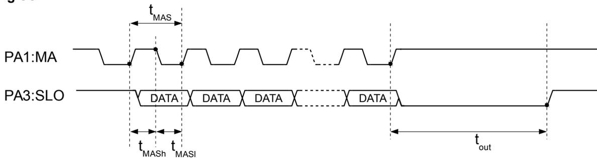
Figure 5: Timing SSI interface (NTOA = 1)
