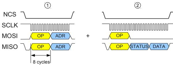
Figure 29: Read REGISTER (single): set the read address (1) + command REGISTER status/data to read-out data (2)
