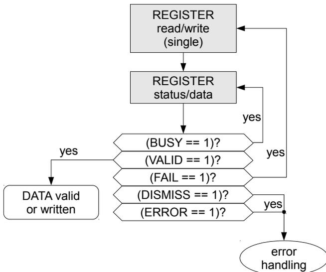
Figure 32: Example sequence of commands REGISTER read/write and REGISTER status/data
