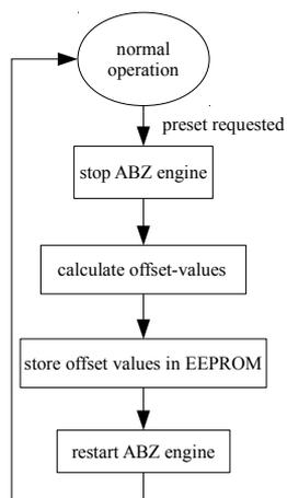
Figure 55: Preset sequence using command
