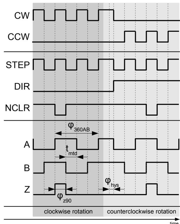
Figure 45: Definition of the ABZ, STEP/DIR, and CW/CCW signals
