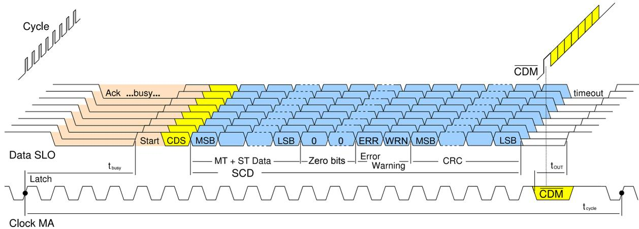
Figure 17: Example of BiSS line signals
