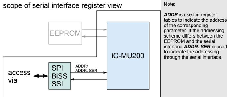
Figure 49: Scope of register mapping serial interface
