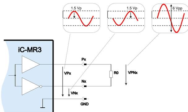
Figure 11: Output signals in mode Analog 1.
