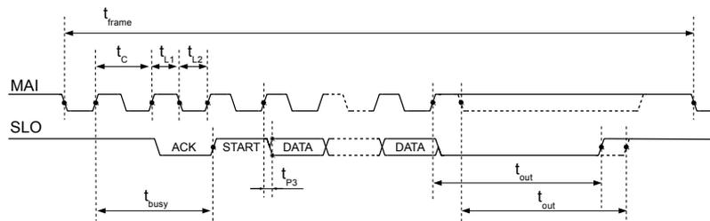
Figure 7: BiSS C protocol timing (ACQMODE  $\neq$  00)
