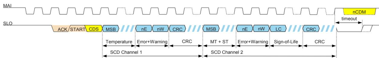
Figure 32: Example of line signals (BiSS C)
