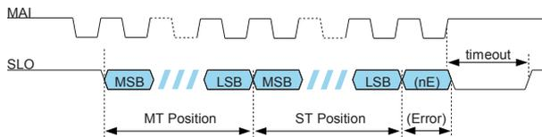
Figure 33: Example of line signals (25-bit Std. SSI)
