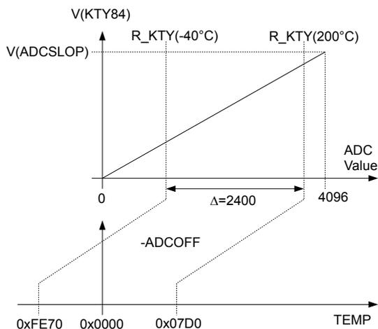
Figure 16: Calibrating the temperature sensor to the output format
