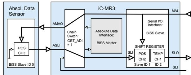
Figure 26: ADI operated in BiSS chain. iC-MR3 now occupies slave ID 1 and 2.
