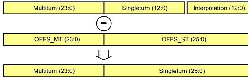
Figure 20: Position data generation with offset correction
