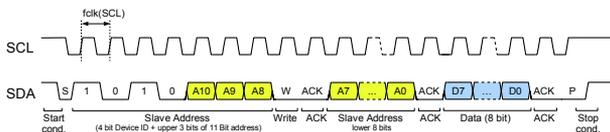
Figure 37: I<sup>2</sup>C slave addressing for writing a single byte to the EEPROM.
