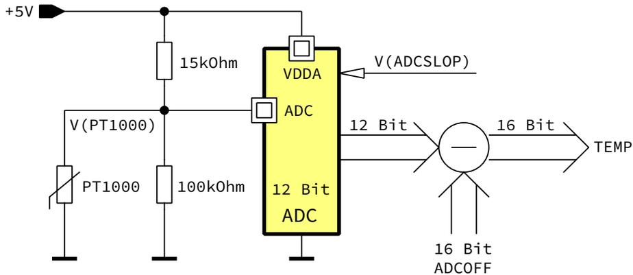
Figure 17: Schematic circuit diagram for the evaluation of PT1000 sensors.
