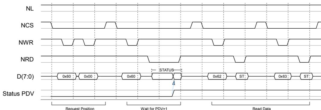
Figure 30: Position data output at request by command
