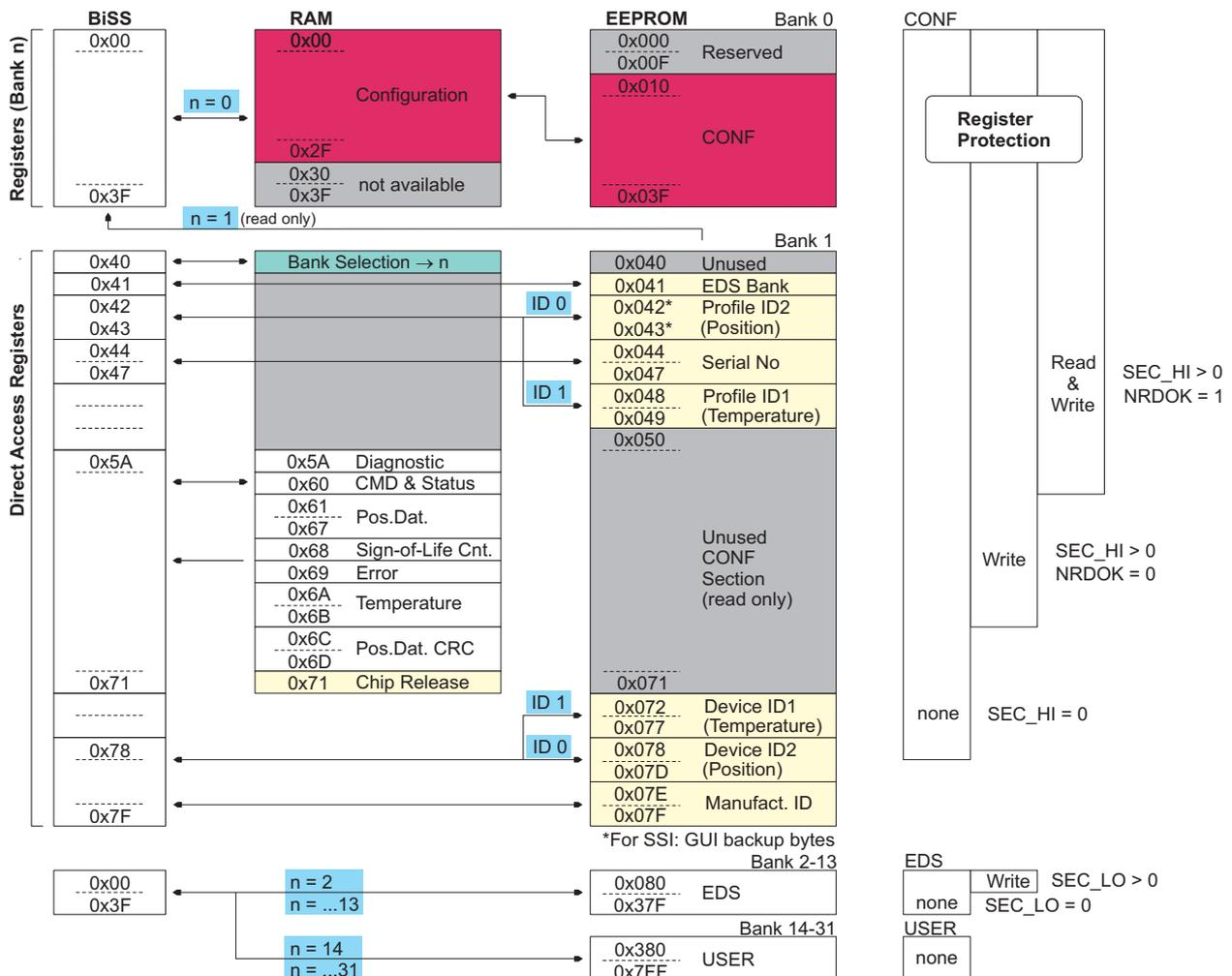
Figure 38: Bankwise memory addressing via BiSS. Example uses CFG\_E2P = 0x2 for a 16 Kbit EEPROM.
