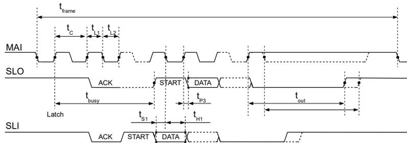
Figure 8: BiSS C protocol timing with triggered conversion (ACQMODE = 00) and chain operation
