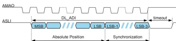
Figure 23: ADI data frame with SSI protocol
