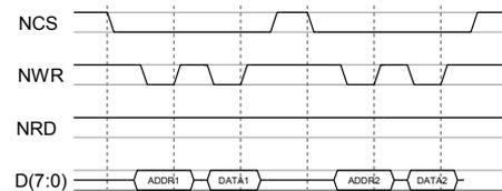
Figure 29: Write process
