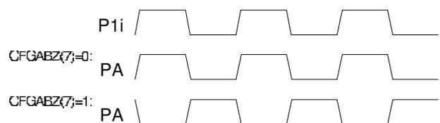
Figure 14: Function of CFGABZ(7)
