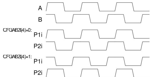
Figure 13: Function of CFGABZ(4)
