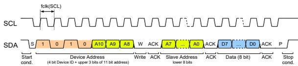
Figure 2: I<sup>2</sup>C slave addressing for writing a single byte to the EEPROM.
