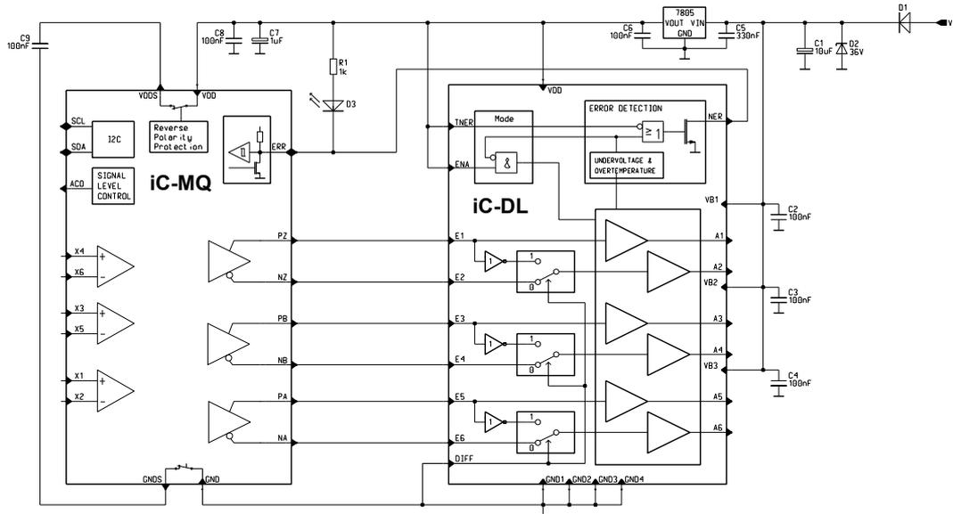
Figure 29: Application example with 24 V line driver.
