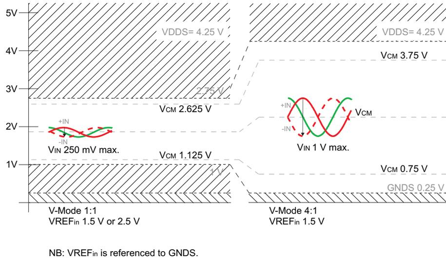
Figure 5: Permissible common mode range and maximum input signal at lowest gain (GR12= 0x0, GF1, GF2 = 0x00); left side: voltage input 1:1, right side: voltage input 4:1.
