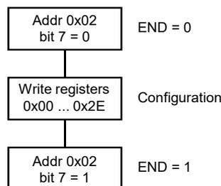
Figure 3: Programming via I<sup>2</sup>C. END is altered by changing only bit 7 of address 0x02 and leaving bits 6:0 unchanged.
