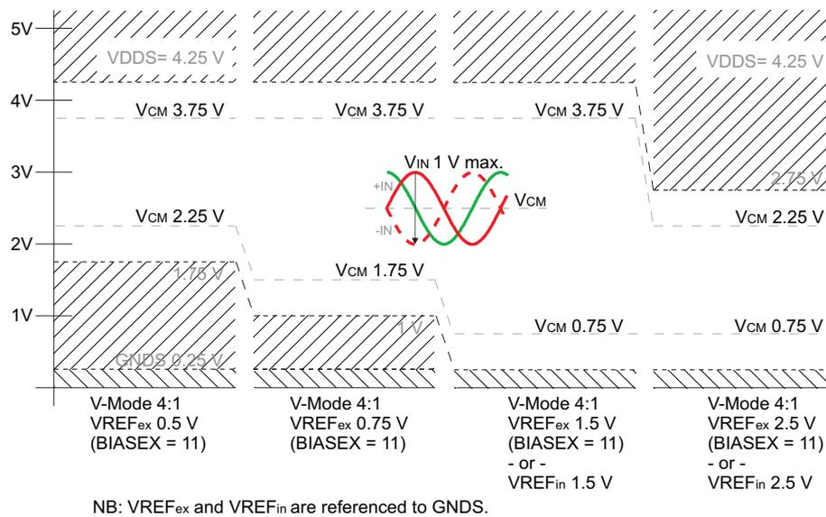
Figure 6: Permissible common mode range for voltage input 4:1 in dependency to the reference voltage.
