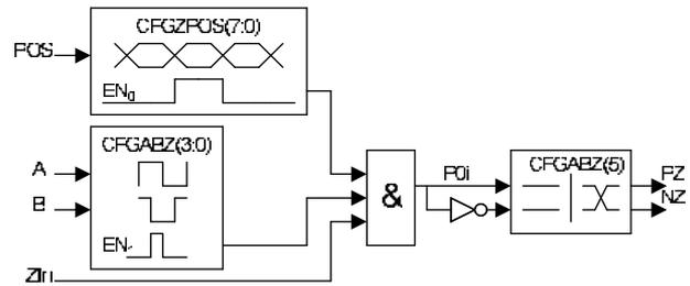
Figure 11: Signal path from  $Z_{in}$  to PZ/NZ
