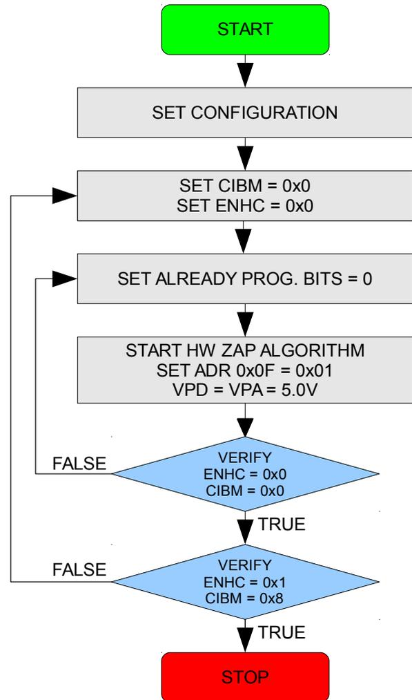
Figure 30: Programming algorithm
