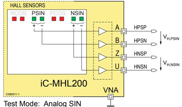
Figure 12: Output signals of the sine Hall sensors in test mode Analog SIN
