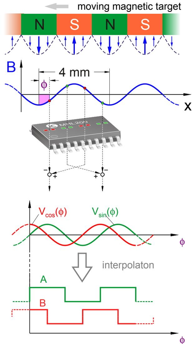
Figure 7: Signal generation and position data output
