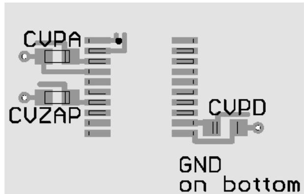
Figure 32: Example PCB layout for the TSSOP package
