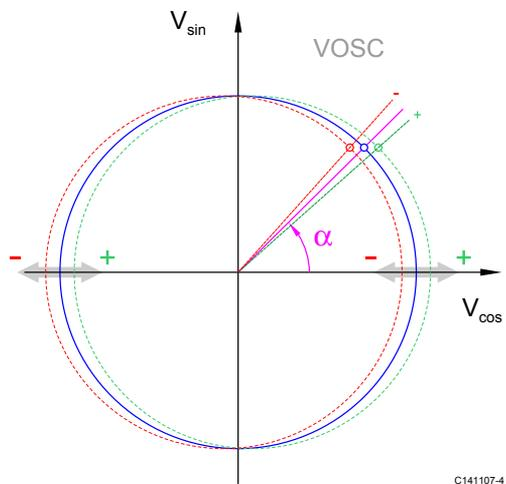
Figure 19: Effect of the cosine offset setting
