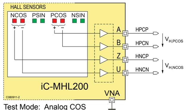
Figure 13: Output signals of the cosine Hall sensors in test mode Analog COS
