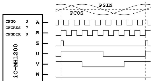
Figure 27: ABZ incremental signals / period counter
