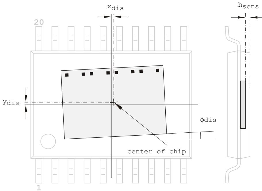
Figure 3: Definition of lateral and rotational displacements
