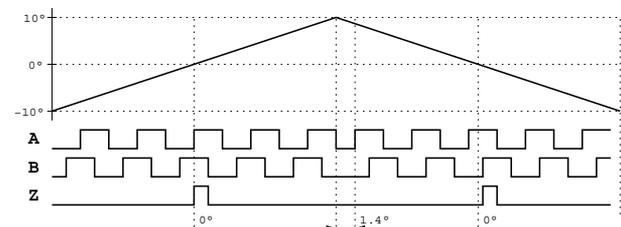
Figure 23: Quadrature signals for rotating direction reversal (hysteresis 1.4 °)
