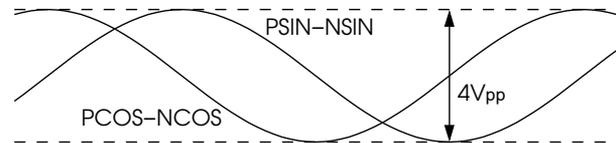
Figure 11: Definition of differential amplitude
