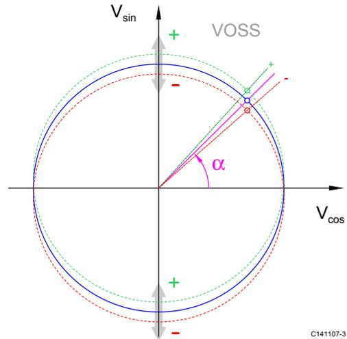
Figure 18: Effect of the sine offset setting
