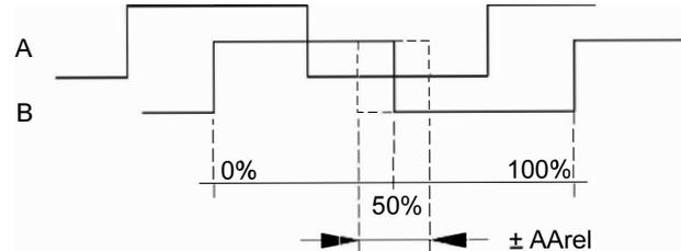
Figure 22: ABZ signals and relative accuracy
