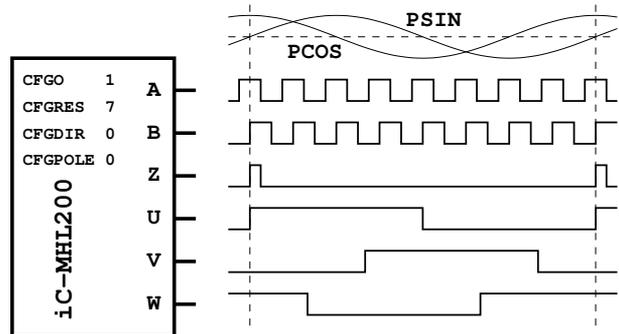
Figure 25: ABZ incremental / UVW commutation signals
