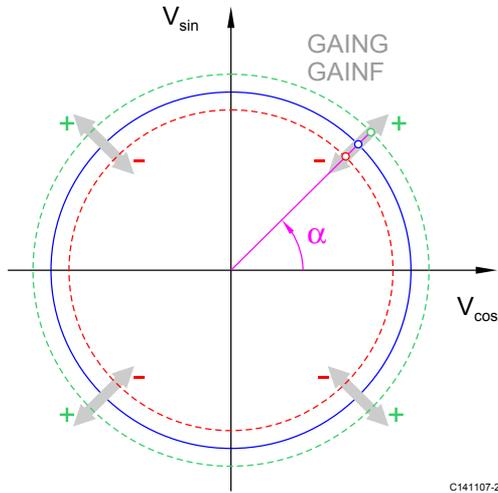
Figure 17: Effect of gain settings GAING and GAINF
