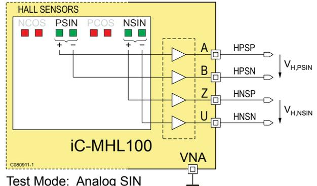
Figure 8: Output signals of the sine Hall sensors in test mode Analog SIN
