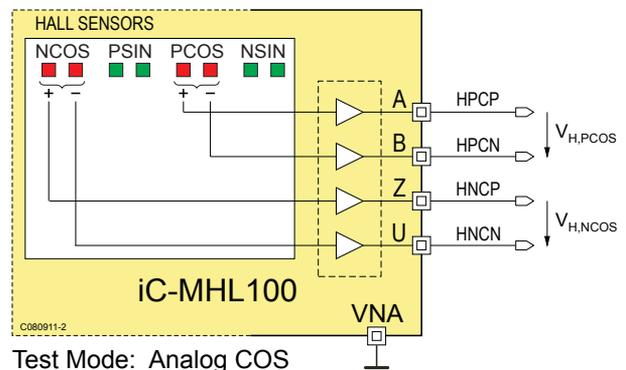
Figure 9: Output signals of the cosine Hall sensors in test mode Analog COS
