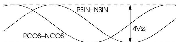
Figure 7: Definition of differential amplitude
