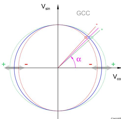
Figure 16: Effect of the amplitude ratio
