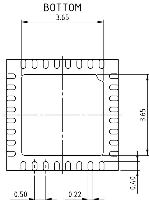
All dimensions given in mm. Tolerances of form and position according to JEDEC MO-220.
