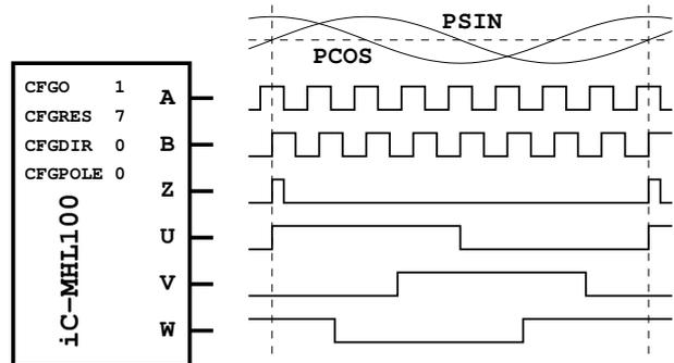
Figure 21: ABZ incremental / UVW commutation signals
