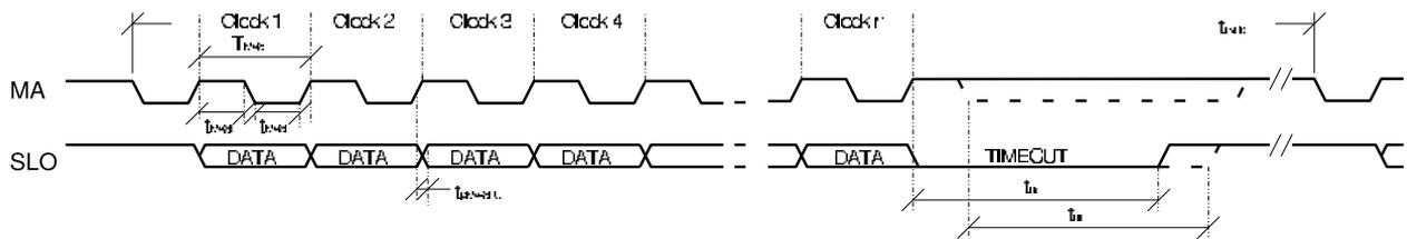
Figure 1: Serial Interface timing with SSI protocol
