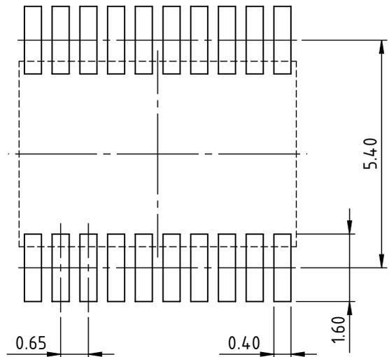
All dimensions given in mm. Tolerances of form and position according to JEDEC MO-153.
