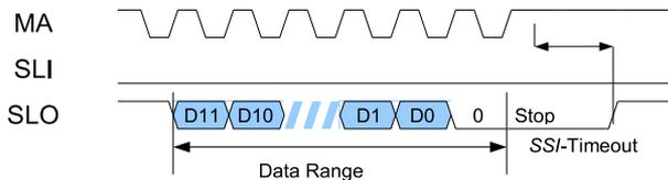
Figure 25: SSI protocol, data GRAY-coded
