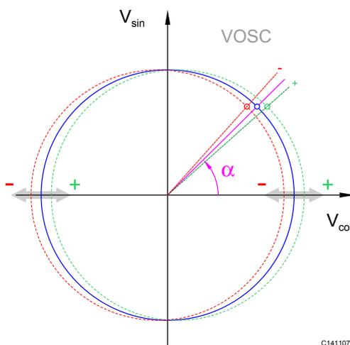
Figure 15: Effect of the cosine offset setting
