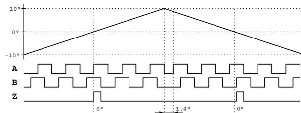
Figure 19: Quadrature signals for rotating direction reversal (hysteresis 1.4 °)
