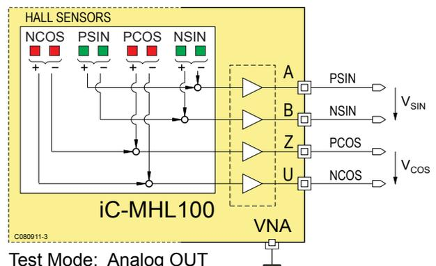
Figure 10: Differential sine and cosine signals in test mode Analog OUT
