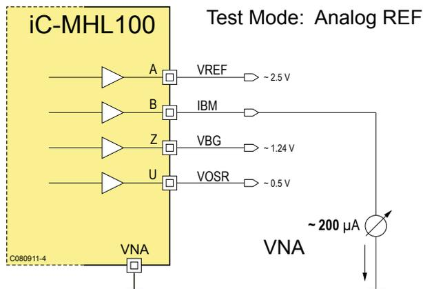
Figure 11: Setting bias current IBM in test mode Analog REF
