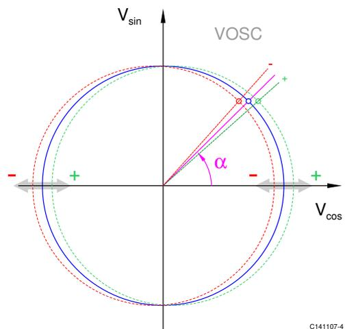
Figure 16: Effect of the cosine offset setting
