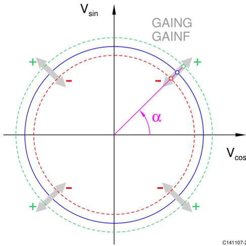
Figure 14: Effect of gain settings GAING and GAINF
