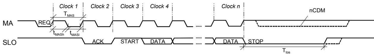
Figure 2: Timing diagram in BiSS C protocol.
