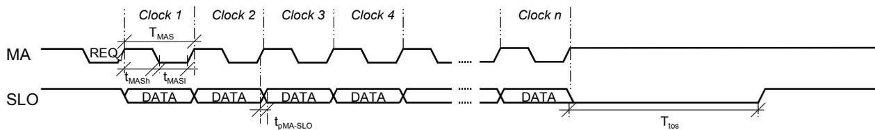
Figure 1: Timing diagram in SSI protocol.
