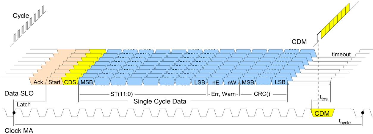
Figure 24: Example line signals (BiSS C)
