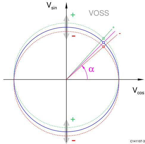
Figure 15: Effect of the sine offset setting
