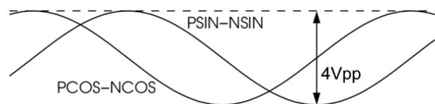
Figure 7: Definition of differential amplitude
