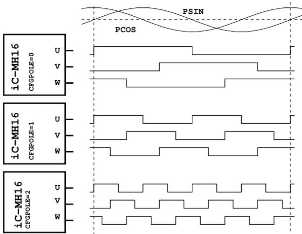
Figure 22: UVW signals for different settings of CFG-COM
