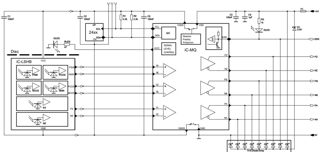
Figure 1: Example of incremental encoder with RS422 output
