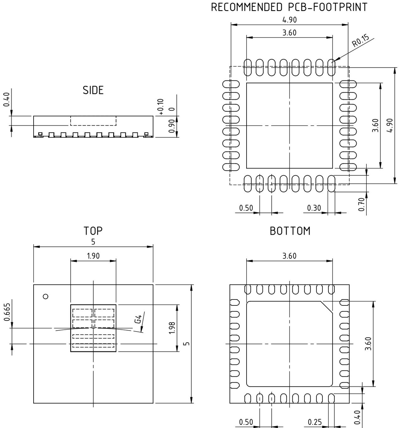
All dimensions given in mm. General Tolerances of form and position according to JEDEC MO-220.
