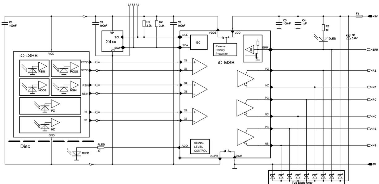
Figure 2: Example of sine encoder with 1 Vpp output
