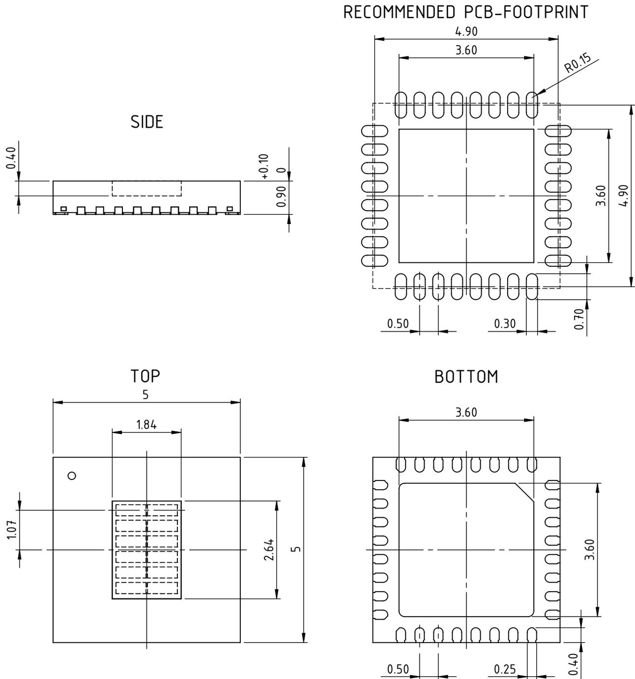
All dimensions given in mm. General Tolerances of form and position according to JEDEC MO-220. Positional tolerance of sensor pattern:  $\pm 70\mu\text{m}$  /  $\pm 1^\circ$  (with respect to center of backside pad). Maximum molding excess  $+20\mu\text{m}$  /  $-75\mu\text{m}$  versus surface of glass. Small pits in the mold surface, which may occasionally appear due to the manufacturing process, are cosmetic in nature and do not affect reliability.
