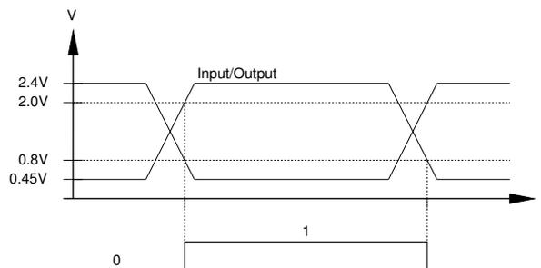
Figure 1: Reference levels for delays
