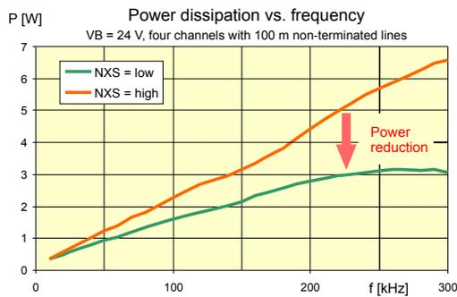
Figure 8: Power dissipation with and without xSwitch-Mode
