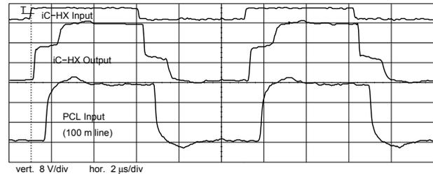
Figure 3: Reflections caused by a mismatched line termination
