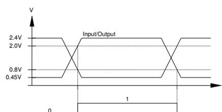
Figure 1: Reference levels for delays
