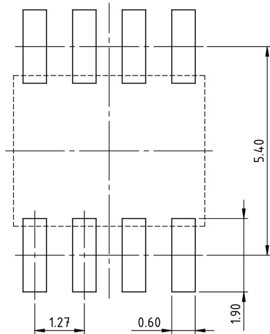
All dimensions given in mm. Tolerances of form and position according to JEDEC MS-012.
