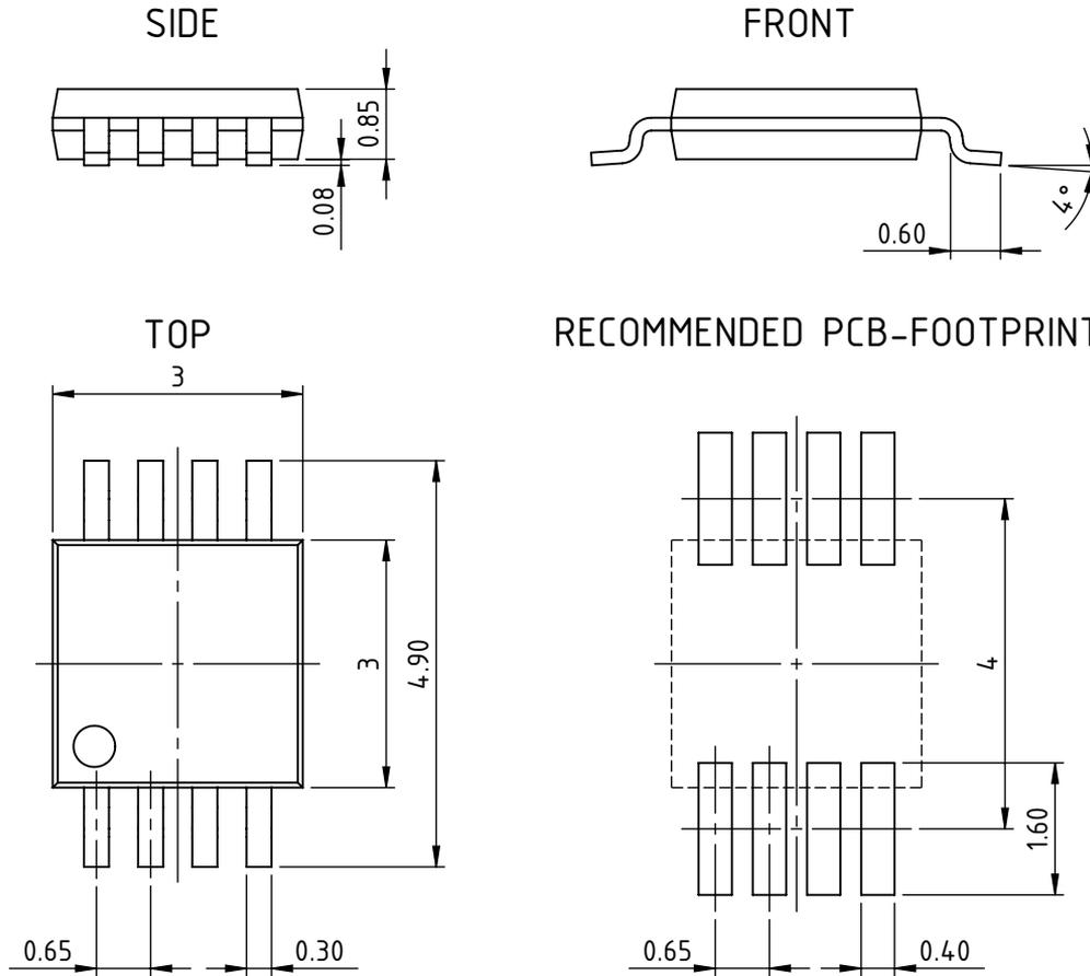
All dimensions given in mm. Tolerances of form and position according to JEDEC MO-187.
