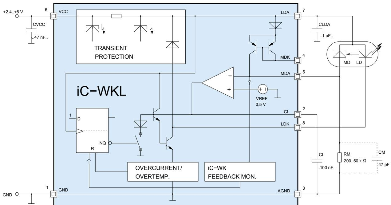
suitable laser diode configurations: N, P, M
