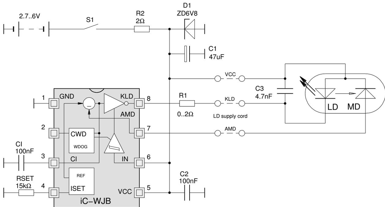
Figure 10: CW operation via cable plus protective circuitry
