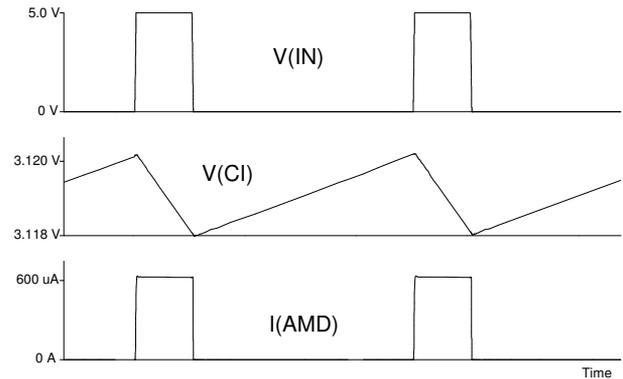
Figure 4: Steady-state APC,  $f(IN) = 100 \text{ kHz}$  (1:4),
