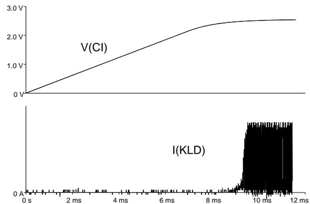
Figure 5: Turn-on behaviour,  $f(IN) = 100 \text{ kHz}$  (1:1),
