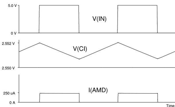
Figure 3: Steady-state APC,  $f(IN) = 100 \text{ kHz}$  (1:1),
