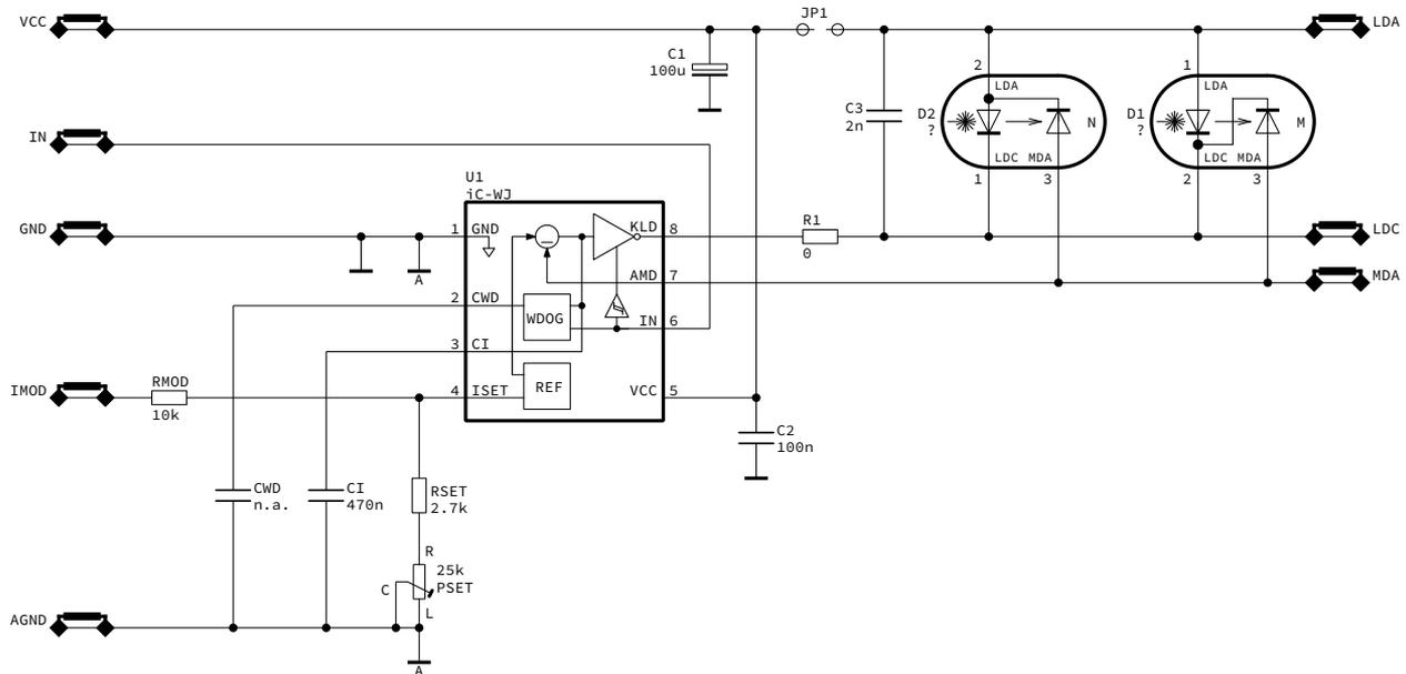
Figure 12: Schematic diagram of the Demo Board
