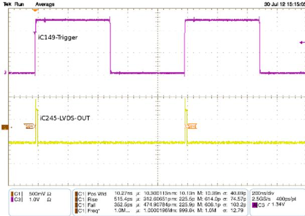
Figure 7: Maximum pulse width of 10.2 ns
