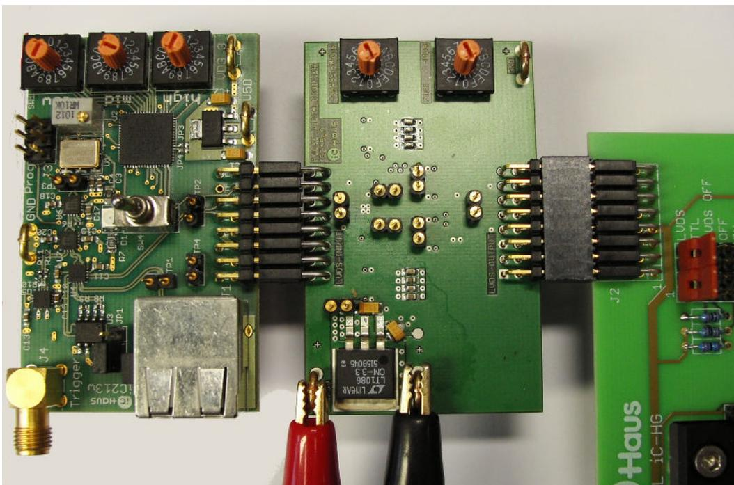
Figure 6: Connecting iC213 and iC245 to HG2D.
