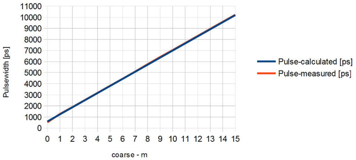
Figure 3: Setting the pulse width "coarse"
