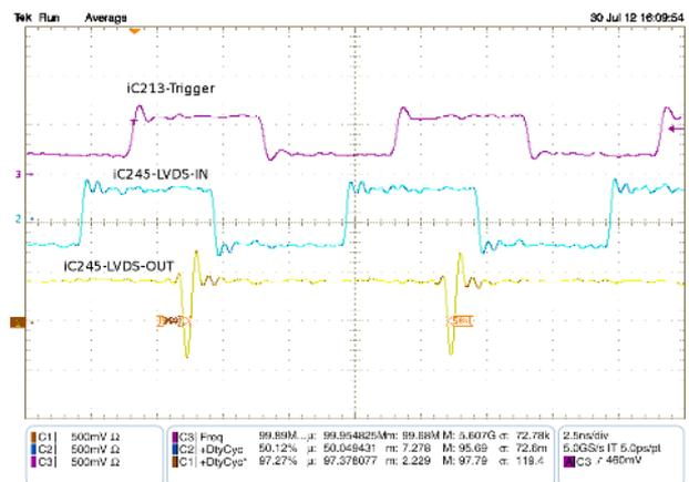
Figure 12: 100 MHz signal from iC213 and a long duty cycle > 97%
