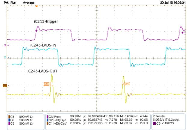
Figure 10: 100 MHz signal from iC213 and a short duty cycle < 3%
