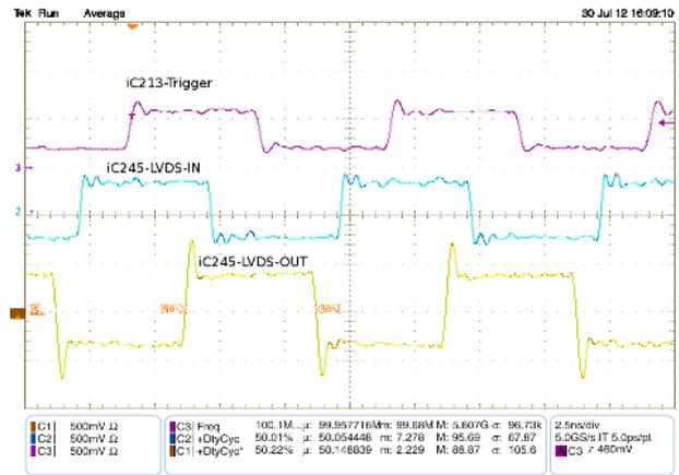
Figure 11: 100 MHz signal from iC213 and a duty cycle of 50%
