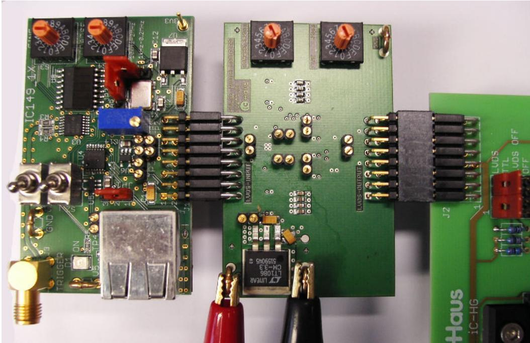
Figure 5: Connecting iC149 and iC245 to HG2D.
