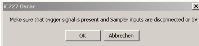
After pressing the OK button the offset of CH1 and CH2 are set to zero.
