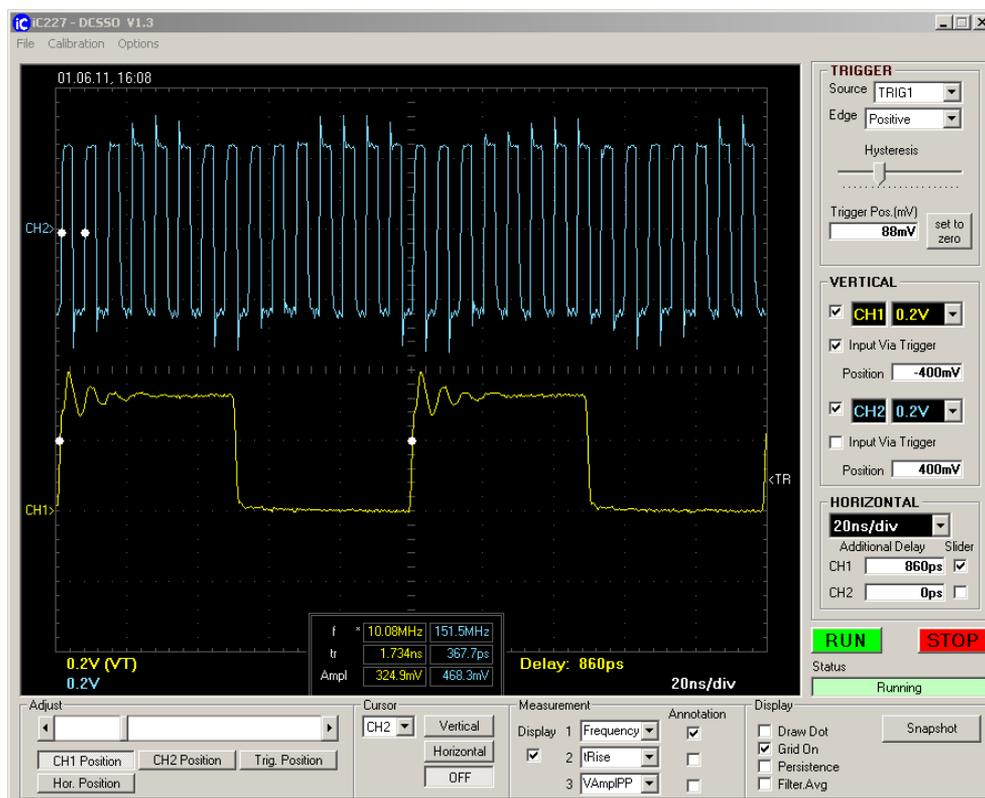
Figure 44: RF generator output frequency 150 MHz
