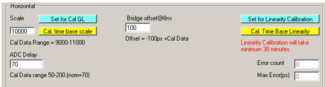
Figure 31: Horizontal calibration
