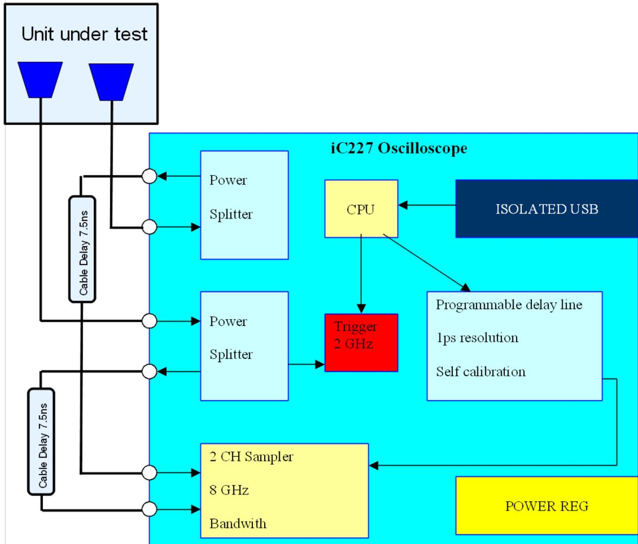
Figure 3: 4 GHz Setup
