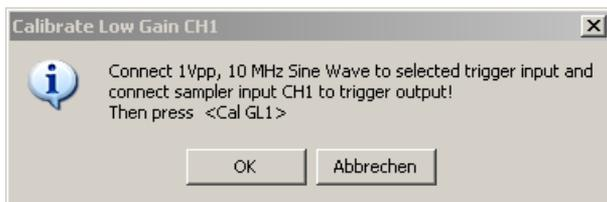
Figure 28: Amplitude calibration
