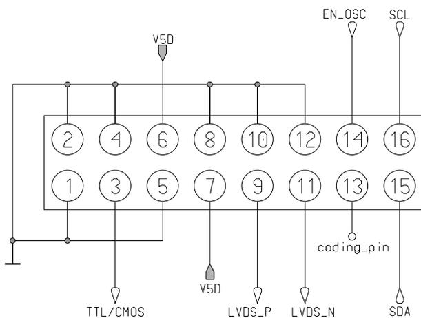
Figure 2: Pin configuration J1 (PCB bottom view)
