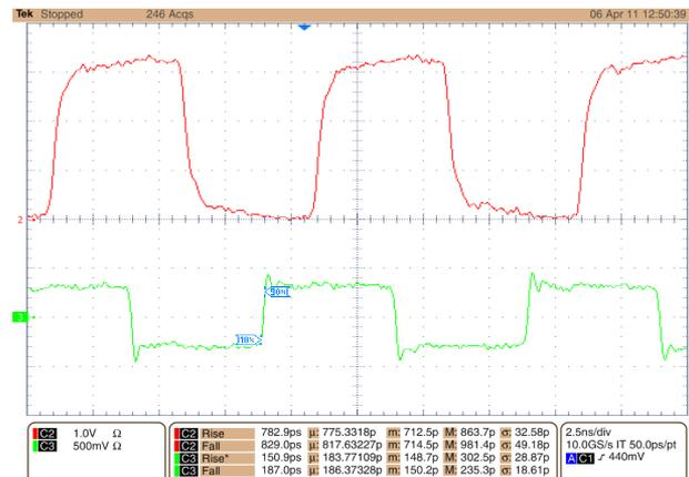
Figure 3: Channel 2 (red) TTL output, Channel 3 (green) LVDS Output
