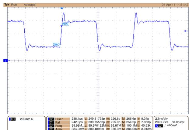
Figure 4: Channel 1 (blue) trigger signal with 100 MHz
