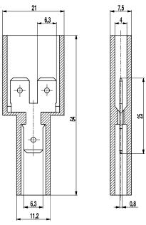
Tab connector 406 is only available as 1-pole variant. It features one single connection  $6.3 \, \text{mm}$  on one side and a double connection  $2x6.3 \, \text{mm}$  on the opposite side.
