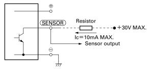
Output waveform(Need pull-up resistor) In case of steady running
