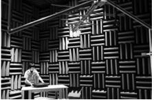
Acoustic radio wave anechoic chamber
