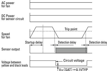
Example 2: When the AC power for the fan is turned on first, then the DC power for sensor is powered on
