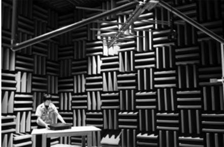
Acoustic radio wave anechoic chamber
