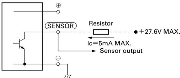
**Output waveform** (Need pull-up resistor)
