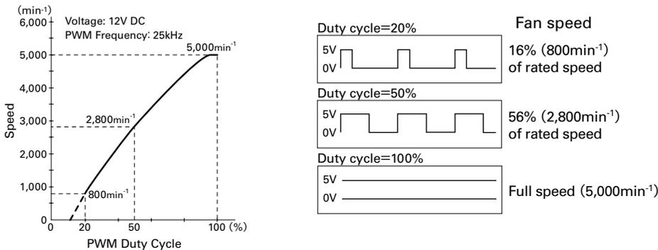
The dotted part of the performance curve (area below 20% PWM duty cycle in the above case) indicates the fan speed is unstable in the area.
