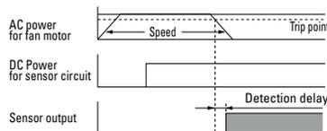
Example 3: When the DC power for sensor is first powered on, then the AC power for the fan is turned on
