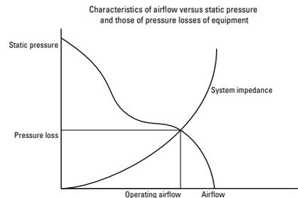
Since the value obtained from the above equation is only a rough target, final fan selection should be based on your actual installation test.
