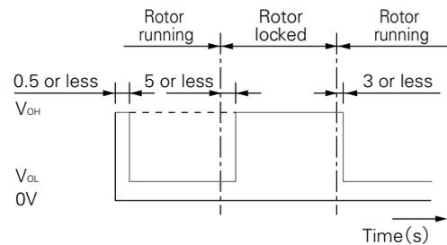
Note: The output is completely at  $V_{OL}$  with 0.5s or less after power-up.
