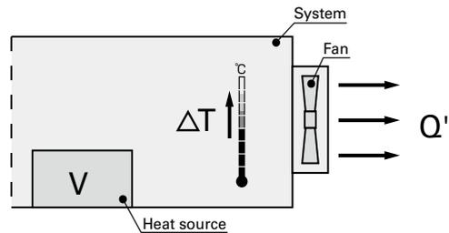
**2. Calculating the required airflow for cooling**
