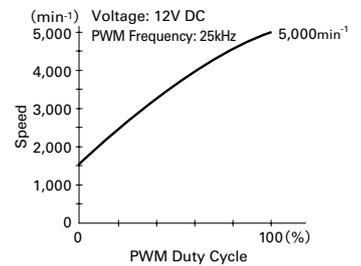
Controlling device that easily regulates the rotational speed of PWM control fans function
