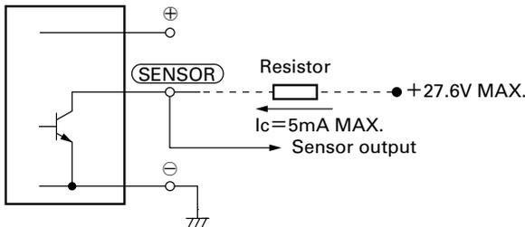
**Output waveform** (Need pull-up resistor)
