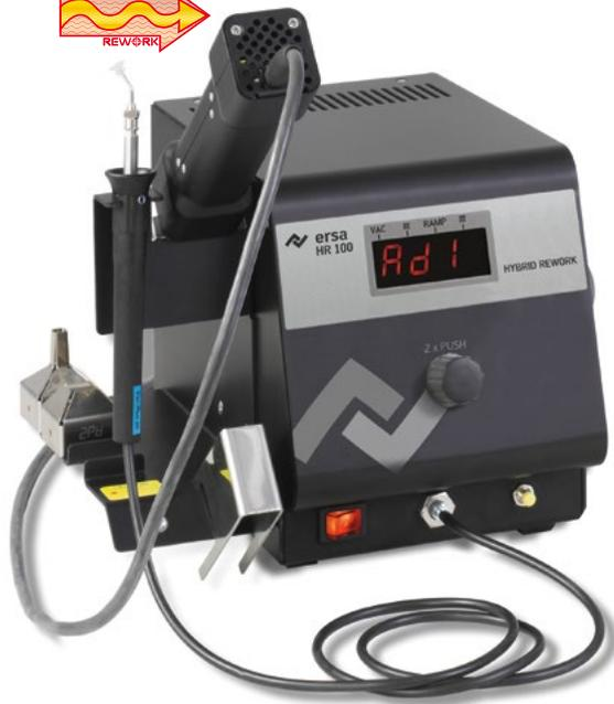
The **HR 100 A** uses Ersa's revolutionary and patented Hybrid Rework Technology for safe removal and replacement of small SMDs in a lead-free environment. Safe, medium-wave IR radiation combined with a gentle hot air stream guarantees optimal energy transfer to the component.
