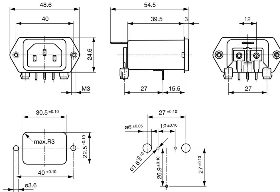
PCB rear side mounting, protection class I
