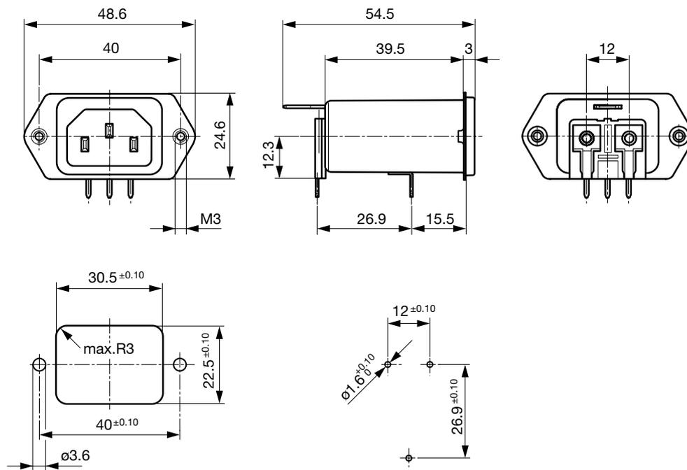
PCB snap-in rear side mounting, protection class II
