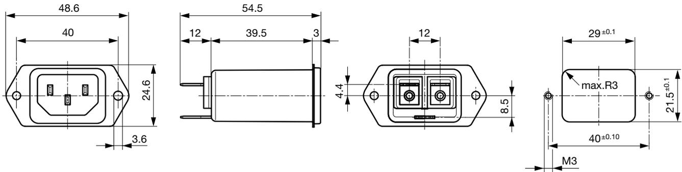
Rear side mounting with pre-formed, threaded holes for M3 screws (panel cutout for rear side mounting)
