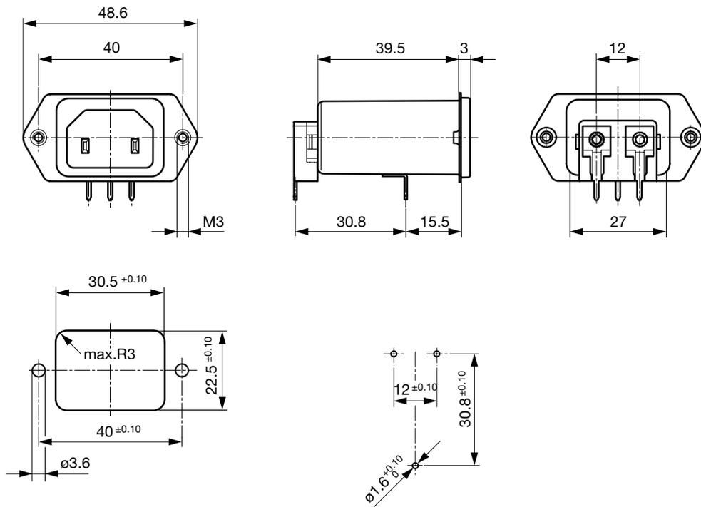
Screw and snap-in mounting with flexible wire
