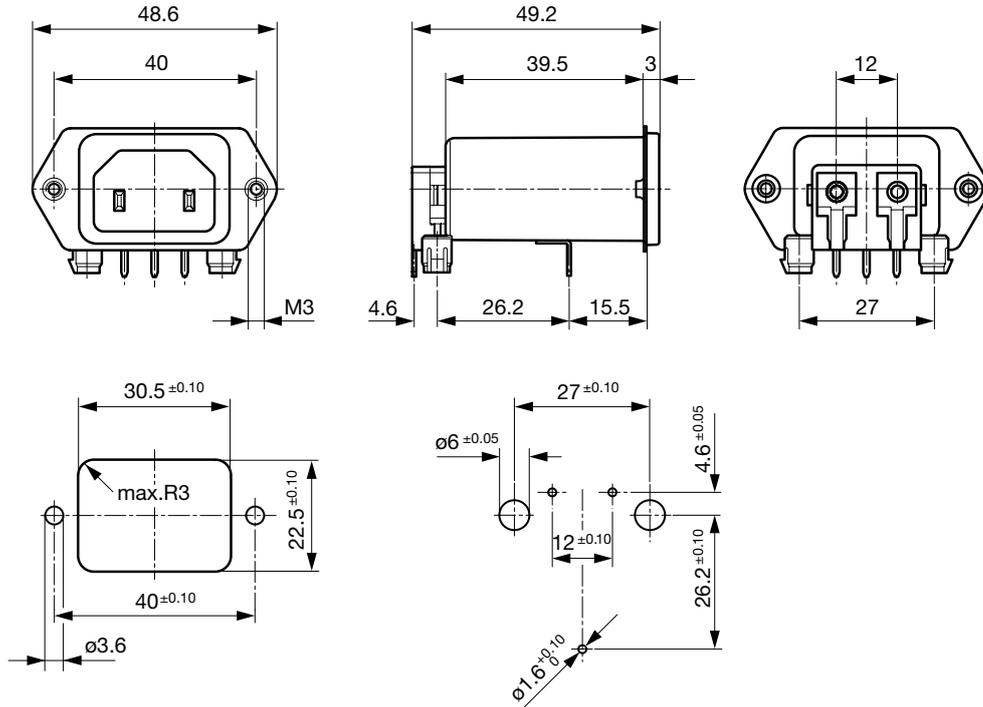
PCB rear side mounting, protection class II
