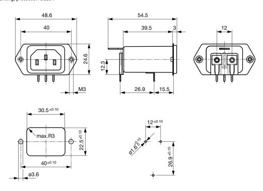
PCB snap-in rear side mounting, protection class II
