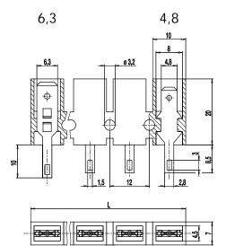
The combined tab/solder connector blocks are used primarily as connectors, cable splitter or as a base in electrical appliances and in automotive.
