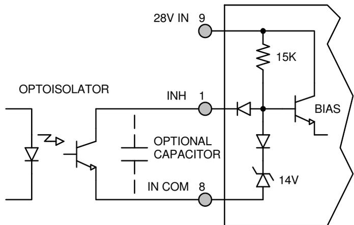
Figure 5 – Isolated Inhibit Drive
